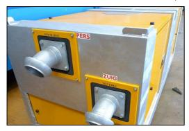
The panels are 2 cm inside in the frame to prevent damaging during transport.
